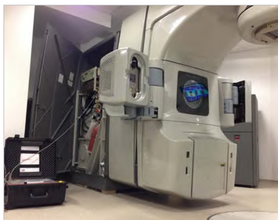
The B160R92 unit is adapted to the requirements of small gas compartments. The photo shows the device during service works on a medical radiation unit.
